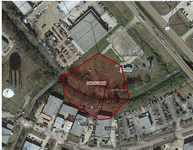
Figure G-18 – 2D Boundary Condition Line for flow into Claycut Bayou near Airline Highway
